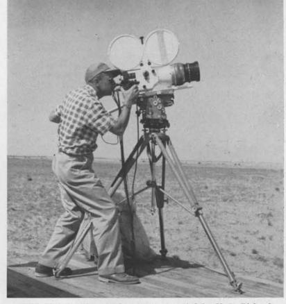
HIGH SPEED 35mm movie camera, operated by N. L. Richardson (5216), provides additional data for study. This camera can take 1500 frames per second. Normal projection speed slows action.
